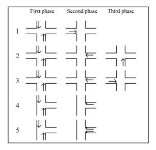
Fig. 4. Arterial intersection phase diagram
