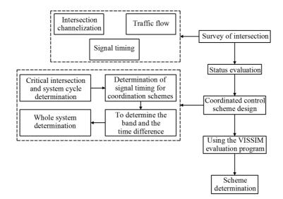
Fig. 2. Signal coordination control system design flow
